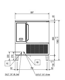
Drain Electrical inlet (power) ΕI Refrigerant Outlet
